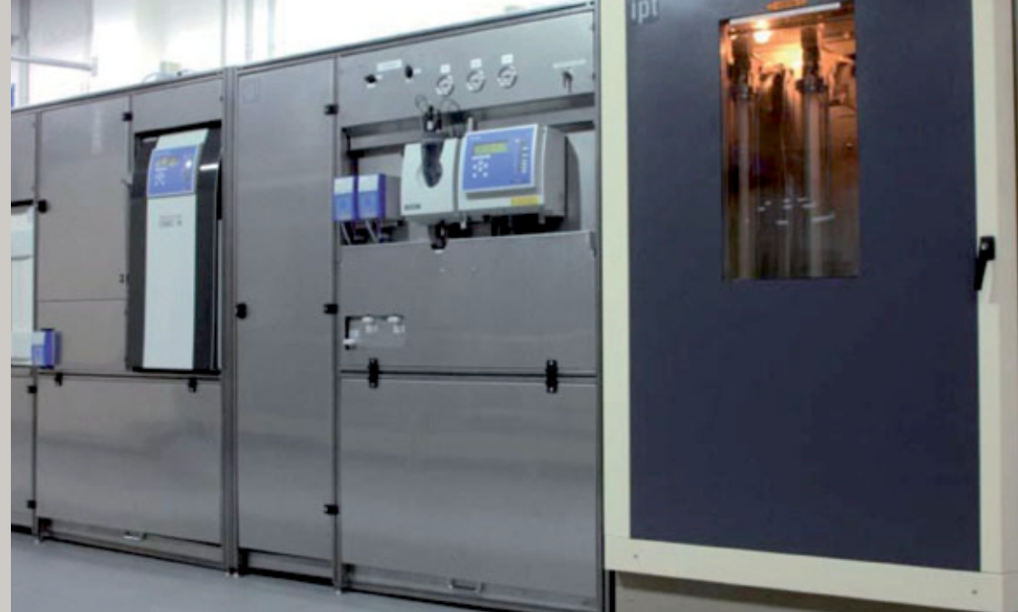
The chlorine test unit
