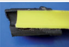
On the left: Mobile Service vehicle - on the right: leak due to incorrect pipe insertion
