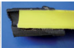
On the left: on-site evaluation – on the right: leak due to incorrect pipe insertion
