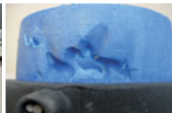
On the left: optical microscope – on the right: flow wear, erosion on a pipe
